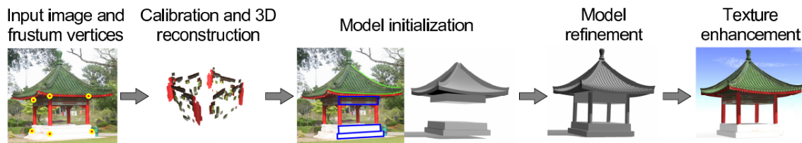
Figure 6: The modeling pipeline. Jiang et al. first calibrate the camera according to the users specified frustum vertices and reconstruct a set of 3D points. The architecture components (i.e. walls and roofs) are then interactively decomposed and modeled. Shape details can be added if necessary. Lastly, the final model is textured with their texture enhancement technique. Content taken from [17].
