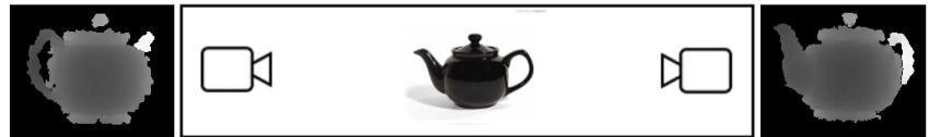
Figure 3: Data acquiring setup. Two Microsoft Kinects positioned opposite of each other for taking the frontal and back view of the object in the middle simultaneously.
