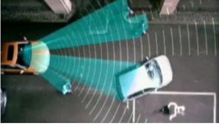
Figure 2: Obstacle detection system in a car for detecting pedestrians and other moving obstacles to help avoiding collisions. 2
