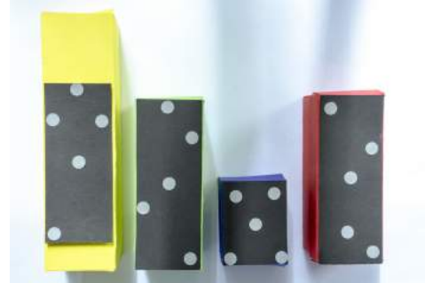
(b) Unique patterns of reflective markers identify the boxes.
