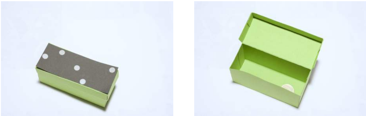
(a) Paper boxes have different lengths and heights expressed in the unit value as well as varying colors. (b) A coin is used to shift the center of mass of each box. It is attached to one of several predefined weight positions.
