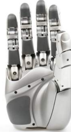
(b) The DLR Hit Hand II is equipped with five identical fingers.
