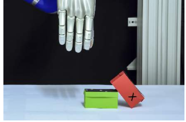
(a) As the weight's position is on the right side of the red box, (b) Positioning the red box at the right edge of the green box is unstable as the weight is on the right.
