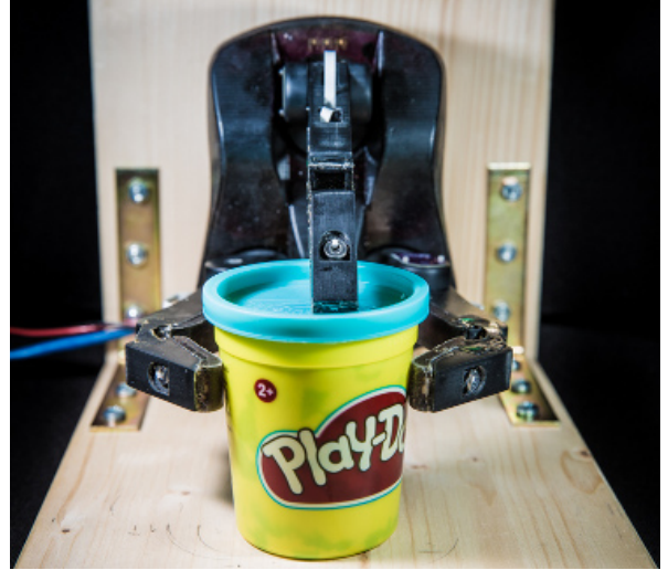
Fig. 1: Using reinforcement learning and tactile feedback, a rolling primitive can be learned on an under-actuated compliant robot hand.
