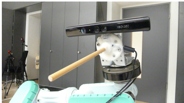
Figure 4.1: The Mitsubishi portable general purpose intelligent arm, PA-10. A 7 degrees of freedom robot arm. Shown while taking an image of a scene to be segmented. The picture on the right shows a close-up view of the robot's "hand" with the end effector and the 3D-camera used, a Microsoft Kinect™
