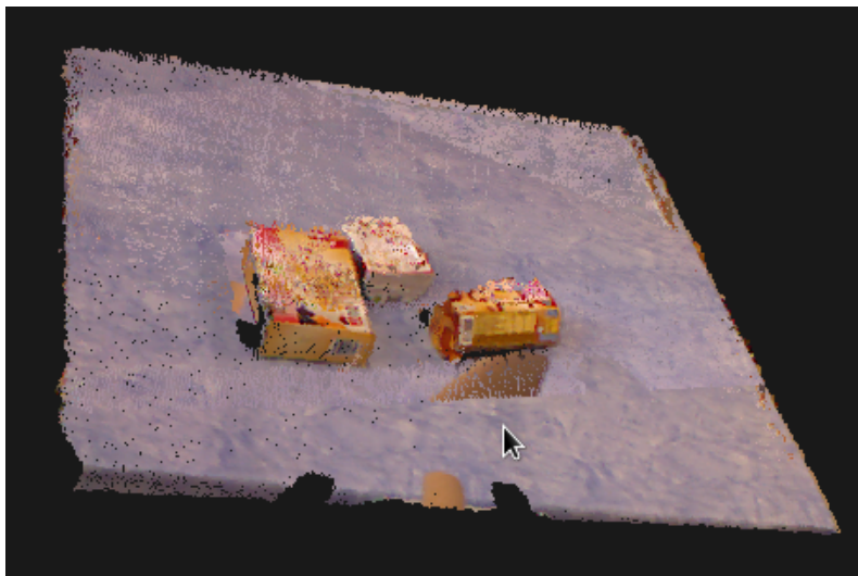
Figure 2.1: Point cloud data recorded by the robot. For every scene, three shots from different directions are taken and combined into one point cloud.
