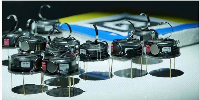
Fig. 1. Kilobots pushing an object in an assembly task. The robots have a diameter of 3.3cm, the object in the background is a square of 1.5cm width.
