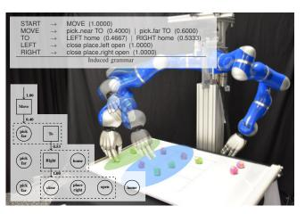
Fig. 1: The robot executes a turn in the tic-tac-toe game, represented as a sequence of movement primitives. The sequence was generated by a probabilistic context-free grammar learned from previously labeled observations.
