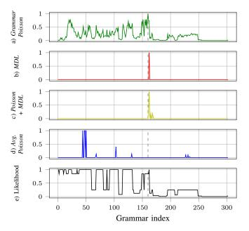
Fig. 7: The posteriors and the likelihood for the box assembly task. The vertical, dashed line indicates the index of the highest posterior (160), given the presented Poisson prior.
